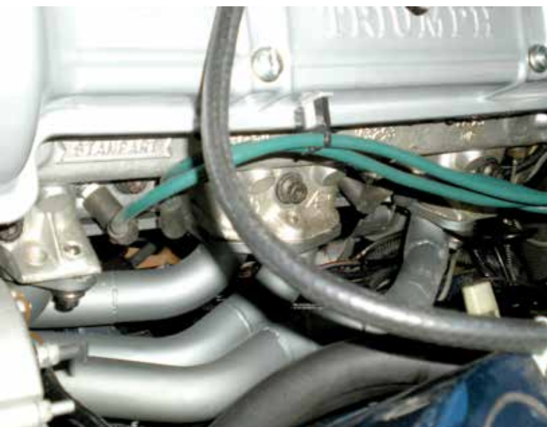
LHS ceramic coated stainless tubular exhaust header. Image: Michael Link
