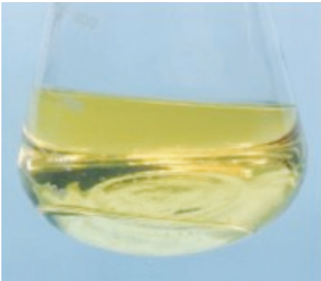
Phase separation can be seen on the right as this ethanol is saturated with water. – graphic courtesy the CTEP project US, DOE
