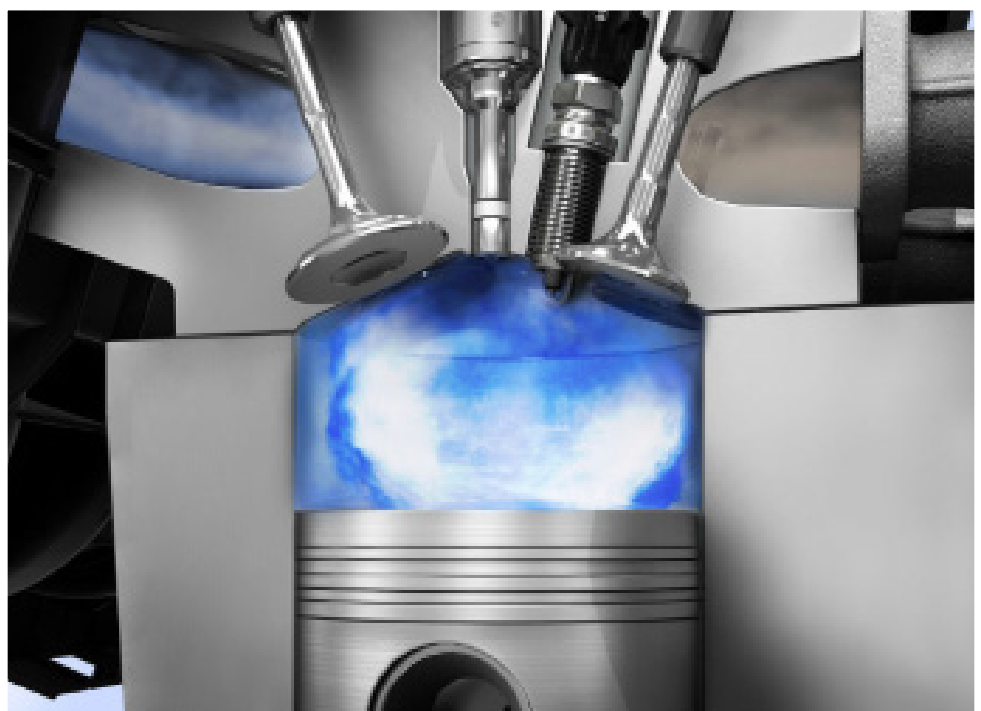
Liquid fuel cannot burn and the cold metal surfaces of the combustion chamber will "quench" the flame of the vaporized fuel that is burning! — Photo courtesy Robert Bosch
